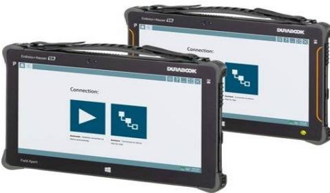
The Field Xpert SMT70 tablet PC for device configuration enables mobile plant asset management in hazardous and non-hazardous areas. It is suitable for commissioning and maintenance staff to manage field instruments with a digital communication interface and to record progress. This tablet PC is designed as a complete solution that comes with pre-installed driver libraries and is an easy-to-use, touch-enabled tool which can be used to manage field instruments during their entire life cycle.
