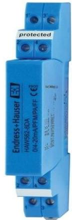
The HAW562 surge arrester is used to protect electronic components from being destroyed by overvoltage. It ensures that overvoltage surges which occur in signal cables (e.g. 4 to 20 mA), in communication lines (fieldbuses) and in power lines are safely passed into the ground. The functionality of the transmitter or the electronics component to be protected is not affected.
