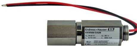
The HAW569 surge arrester is used to protect electronic components in field devices from being destroyed. It ensures that overvoltage surges which occur in signal cables (e.g. 4 to 20 mA), in communication lines of Field buses (HART, PA, FF) and in power lines are safely passed into the ground. The functionality of the electronic component to be protected is not affected as, using the impedance-free connection of the protection unit, interference voltage drops cannot be introduced.
