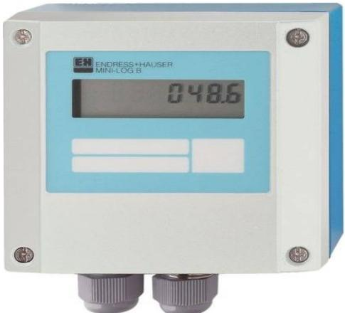
Data logger for stand-alone applications. The Minilog B is used to display and record measured data from an analog and digital input signal. It can be applied where a compact data logger is needed. In addition to data storage the data logger also monitors two set points. Violation of these set values are indicated in the display. Additionally it is possible to transmit a message to a computer or mobile phone using the telephone network or wireless modem (Tele-alarm option).
