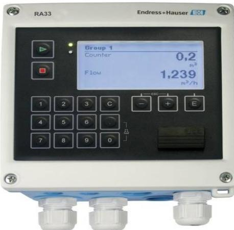
The Batch Controller RA33 is designed to record flow and control output signals for valves and pumps to ensure the exact dosing of predefined batch quantities. The measured volume can be corrected with the temperature/density compensation function. The filling process can be optimized with an automatic or fixed after-run correction. Mineral oils can be corrected according to the ASTM D1250-04 standard.
