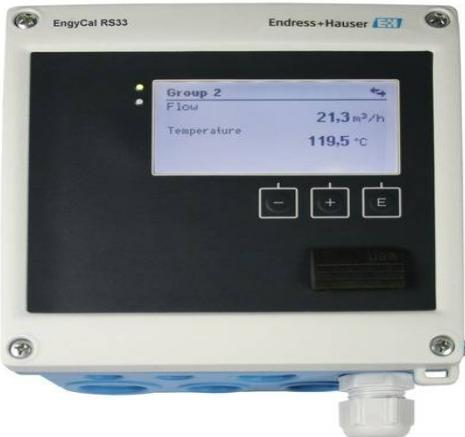
The steam calculator EngyCal RS33 is used to record steam mass and energy flow of saturated and superheated steam. The calculation is based on the measured process variables volume flow, temperature and/or pressure.
