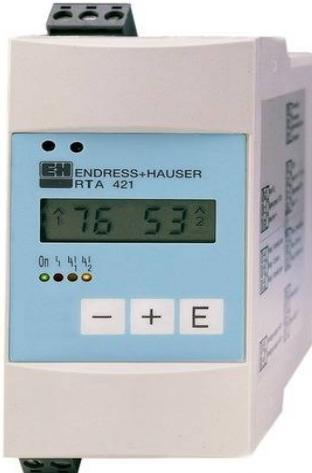
The RTA421 contactor monitors industrial processes for safe operation. The unit analyzes current (0/4...20 mA) and voltage signals (0/2...10 V) and switches two independent output relays if the values either exceed or undercut the preset alarm set points. On the display both limit values are indicated in parallel. The bar graph informs on the connected signal at any time. Applications include pump control in the waste water industry. Level measurement in silos can be economically achieved.
