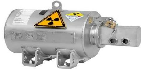
The FQG66 source container is designed to hold the radioactive source with highest activities during radiometric point level detection, continuous level and density measurement. The radiation is emitted almost unattenuated in one direction only, and is damped in all other directions. This guarantees highest safety for the personnel and a reliable measurement.
