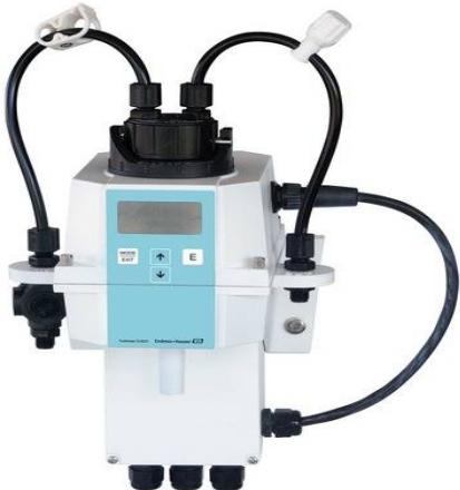
Turbimax CUE21 is a reliable turbidity meter for continuous measurement compliant to EN ISO 7027. Operation is simple: connect the water, adjust the settings and the system runs unattended. Turbimax CUE21 provides guided calibration according to predefined standards, helping to streamline maintenance. Its automatic ultrasonic cleaning function extends service intervals offering significant savings in operational expenditure.
