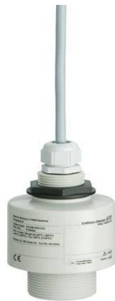
The FDU90 ultrasonic sensor for continuous, non-contact and maintenance-free level measurement of fluids, pastes, sludges and powdery to coarse bulk materials. But also for flow measurement in open channels and measuring weirs. The measurement is unaffected by dielectric constant, density or humidity and also unaffected by build-up due to the self-cleaning effect of sensors. Suited for explosion hazardous areas. Maximum measuring range in liquids 3m (9.8ft), solids 1.2m (3.9ft).
