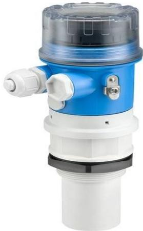
The range of applications extends from monitoring levels in sewage treatment plants and process water tanks to applications for loading, storage and buffer tanks. FMU30 ultrasonic sensor offers proven software algorithms and all warning and alarm messages are shown on the four-line plain text display and guarantee fast remedy of problems. The envelope curve can also be shown on the display. As the analysis results are displayed directly on-site, this ensures quick and accurate error diagnostics.
