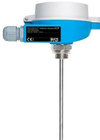
The thermometer is mainly used in the chemical industry but also finds its use in other branches. Preferred applications are vessels or pipes where no high process pressures and no extreme temperatures appear. The device is equipped with a directly wired Pt100-sensor with 4-wire installation. A variety of immersion lengths offers flexible application possibilities.
