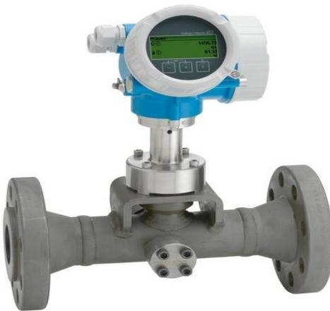
Prowirl C 200 is a product line of carbon steel vortex meters dedicated to the Canadian and American market. The carbon steel sensor offers higher resistance to inter-granular stress corrosion cracking, especially in steam systems for SAGD applications. Prowirl C 200 is only available with cCSAus hazardous area approvals. It is NOT available with CE mark, AD2000 or PED. It is available as compact or remote device version.
