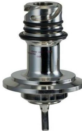
Best applicable for use in hygienic or aseptic pipes and containers or tanks even with very small immersion lengths. It meets increased protection requirements of the temperature sensor regarding physical and chemical effects. Ideally suited to all measuring points that require regular re-calibration by simply replacing the insert in closed processes.
