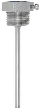
The protection tube is used to match RTD thermometers, such as TST414 from Endress+Hauser, to protect the insert from chemical corrosion. It has a locking screw to fasten the thermometer in place and allows an easy replacement of the thermometer. Due to the reduced wall thickness, it is suggested to use it in processes with slow or medium process flow velocity.
