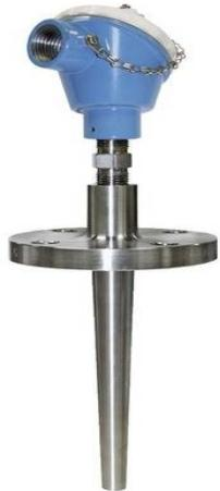
The high modular thermometer is used for several applications with harsh environments, e.g. in power plants, refineries or in the chemical or petrochemical industry. The robust device with barstock thermowell and flange connection in SS316 or INCONEL600 and different head transmitter is a complete unit ready for use with enhanced measurement accuracy and reliability.
