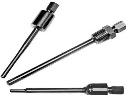
This protection tube is well fitted with an integrated compression fitting, suitable for different industrial applications including even hygienic applications. By default, it is fitted onto pipes and vessels or tanks where attachment to the process can be threaded or welded. Due to its construction various types of temperature probes, such as compact thermometers as well as assemblies without a protection tube or cable probes, generally with a probe diameter of 6 mm, can be applied.
